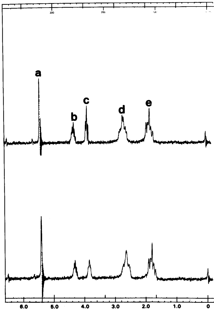
Fig. 1. Proton NMR spectra of 1,7-octadiyne( \text{CuO}_3\text{SCF}_3 ) 2 : a = \text{CH}_2\text{Cl}_2 , b = \text{CD}_3\text{NO}_2 ( \text{CD}_2\text{HNO}_2 ), c = proton on C(1), d = proton on C(3), e = proton on C(4); (above) before addition of \text{CD}_3\text{COOD} , (below) 20 min after addition of one equivalent of \text{CD}_3\text{COOD} .
